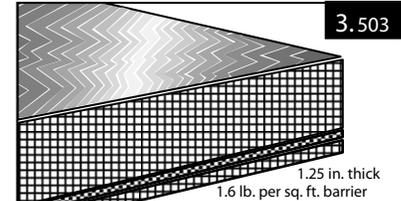
Barymat BTMM-14C – Noise barrier / absorption material with metallized mylar cover and foam decoupler.
