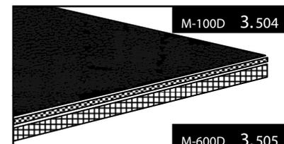
Barymat M-100D – 1.0 lb. per sq. ft. barrier with embossed vinyl wear surface and 0.25 in. foam decoupler.
